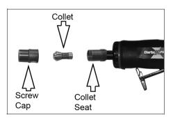
3. If another collet is to be used, undo the screw cap completely and pull out the collet from the collet seat. Replace it with the new collet and screw the cap loosely back on.
